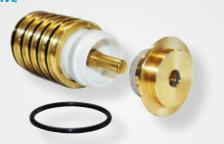
The TF series is equipped with a special, hybrid air valve comprising of a brass body and PET cylinder. The cylinder is made of a light material therefore it does not damage the air valve housing and the pump center body at high pressures.
